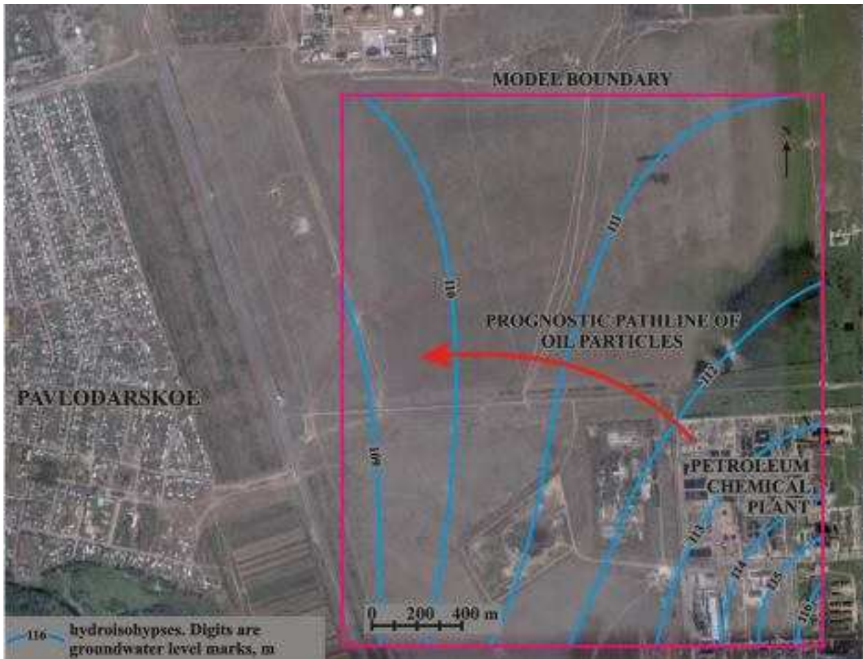
Figure 28. Prognosis trajectory of oil products movement with groundwater (according to results of the modelin
