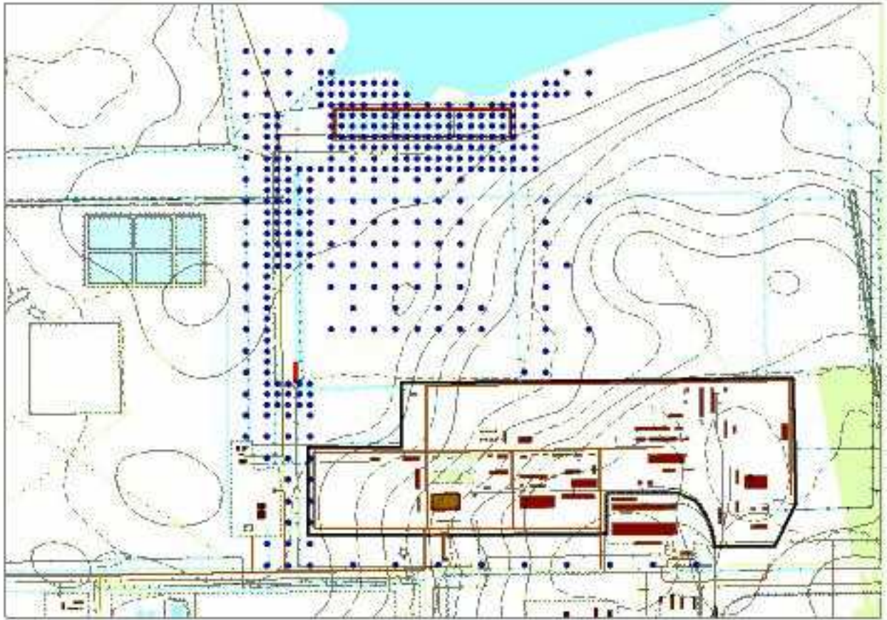
Figure 5. Soil sampling plan from three layers: 0-10, 10-20, 20-50 cm deep at the territory around the industrial site # 1 of PCP
