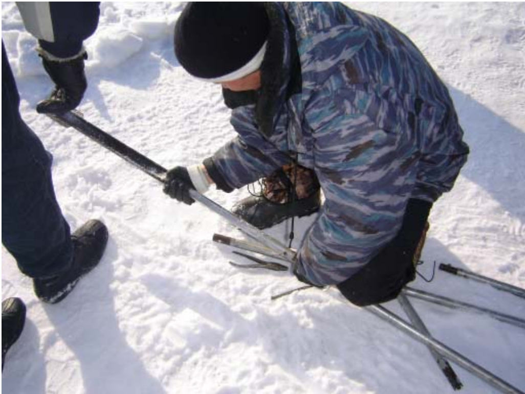
Fig.7. Sampler for level-to-level sampling of soft sediment cores. Wastewater storage pond Balkyldak, March, 2006.
