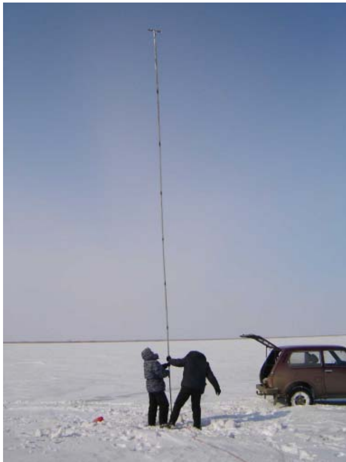
Fig.6. Bottom sediment sampling from the depth of 9 m. Wastewater storage pond Balkyldak, March, 2006.
