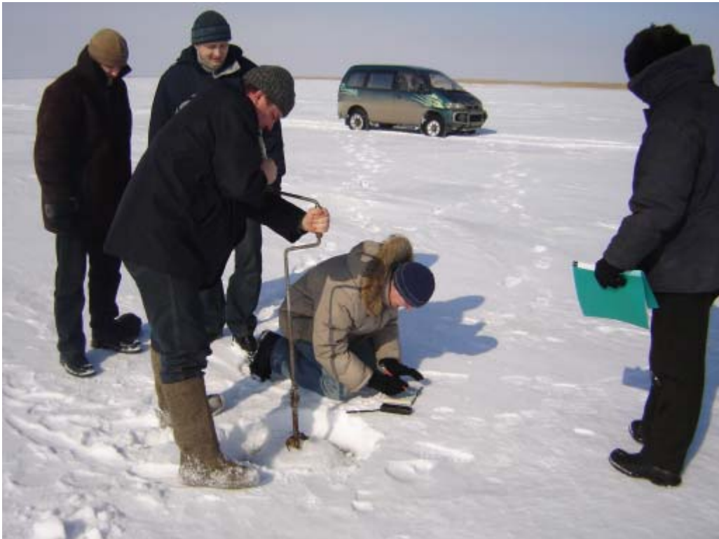
Fig.5. Hole drilling in ice surface in a point of bottom sediment sampling. Wastewater storage pond Balkyldak, March, 2006.
