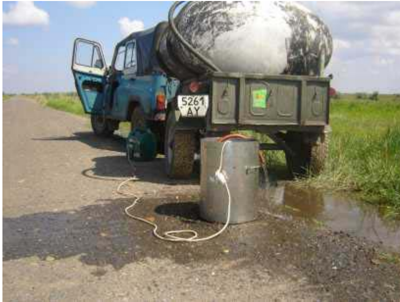
Fig. 5. Equipment rinsing after groundwater sampling
