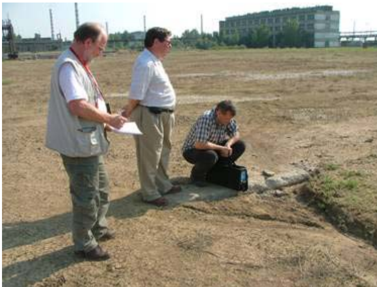
Fig. 7. Measurement of mercury vapors concentration in the near-earth air at the industrial area of chlor-alkali production (in site of the building 31)
