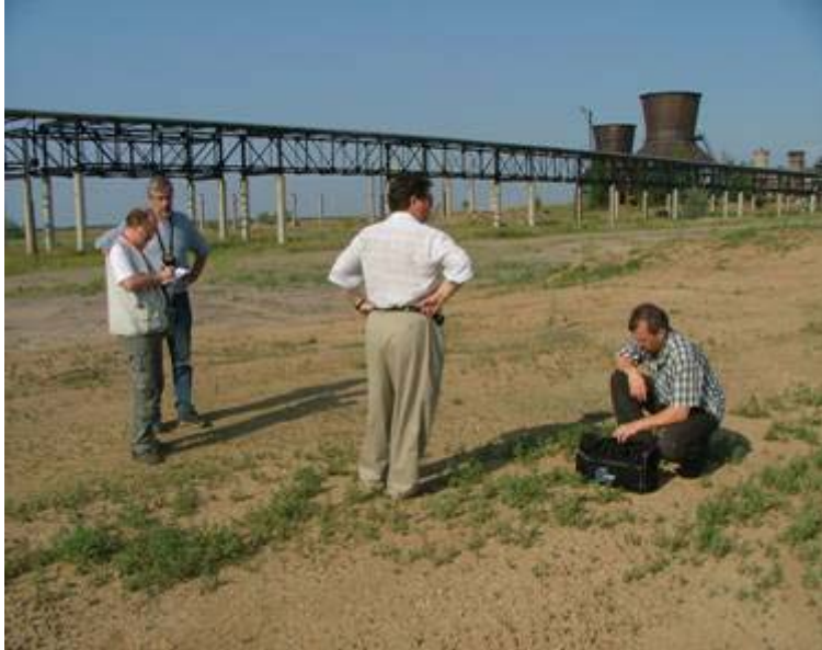
Fig. 8. Measurement of mercury vapors concentration in the near-earth air at the industrial area of the chlor-alkali production (in site of the building 31)
