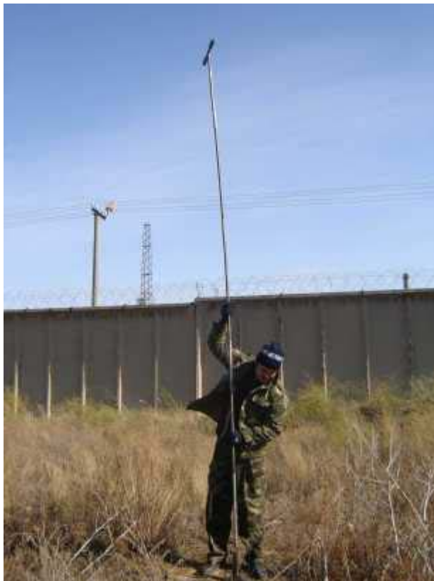
Fig. 11. Drilling of the first test borehole to study spread of oil products pollution near the industrial area of Pavlodfar Oil Refinery
